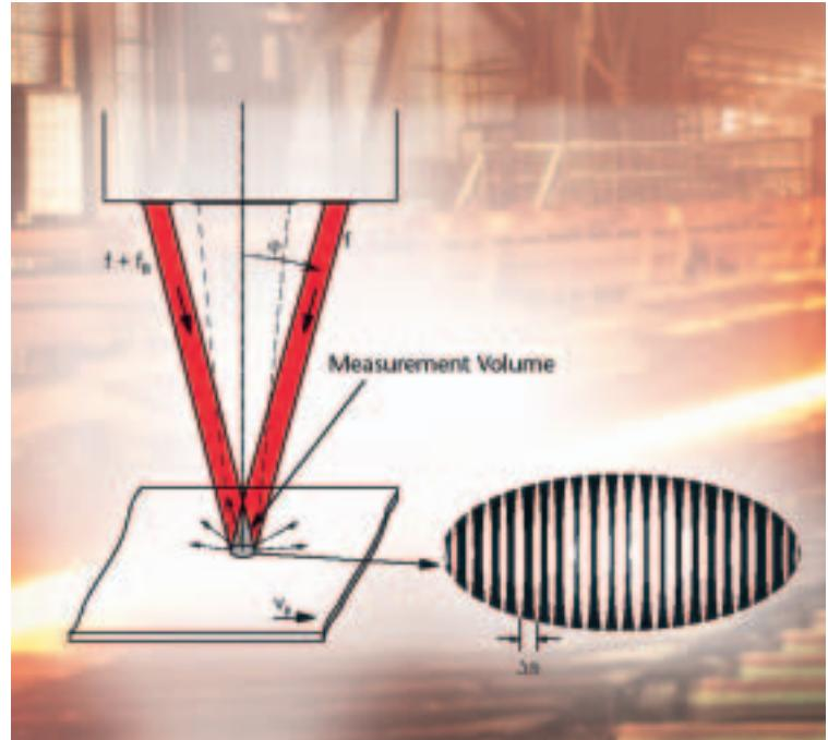
The value  $\lambda / \sin \varphi$  makes up the material measure for the velocity and length measurement.
