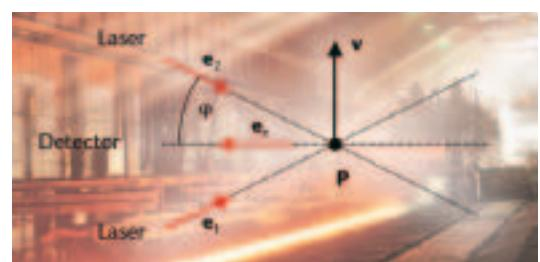
The scatter waves are superimposed on the detector. Due to the interference of the scatter waves from the two laser beams, there are different frequency components in the superimposition. The low-frequency beat frequency of the superimposed scatter radiation which corresponds to the Doppler frequency  $f_D$  is analyzed metrologically. When both incidental laser beams are at the same frequency (same wavelength), this is seen as a difference of  $f_{e2}$  and  $f_{e1}$  to:
