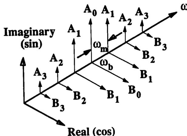
Fig. 2—Frequency components of LDV signal
