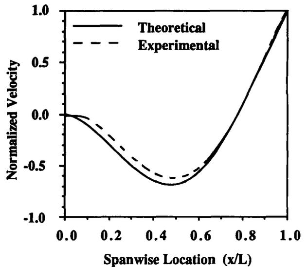
Fig. 6—Beam mode shape (second mode, four terms)
