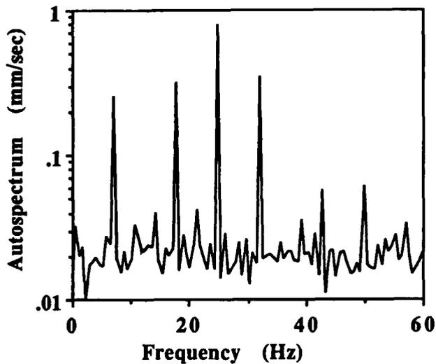
Fig. 4—Autospectrum of scanning LDV output
