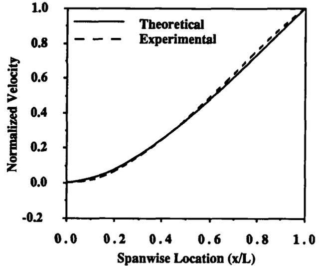
Fig. 5—Beam mode shape (first mode, three terms)
