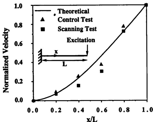
Fig. 3—Beam mode shape (first mode, sorting technique)
