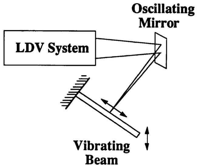
Fig. 1—Scanning LDV experimental setup
