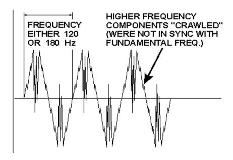
This waveform was detected using either of two different large air core pickup coils:
