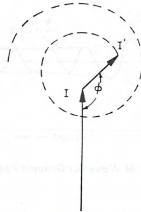
Figure 3-4 (U). Vector Diagram for Changes in Antenna Current
