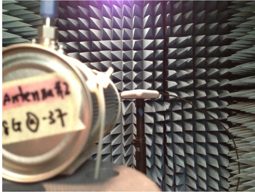
Figure 3.14 Cantenna S21 measurement setup with log periodic antenna
