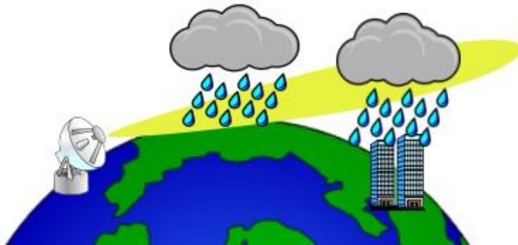
Figure 2.21 Earth’s curvature effect on weather radar
