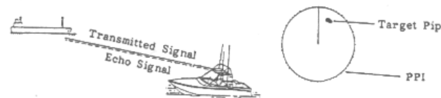
Fig.1 How Radar Works
