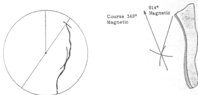
Fig.38 Position Fixing Using Range and Bearing to a Point of Land
