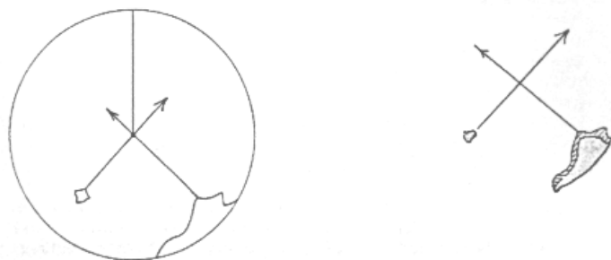
Fig.39 Position Fixing Using Two Bearings
