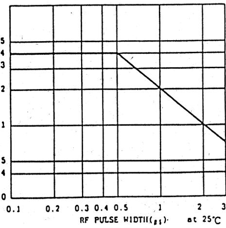
FIG. 2. PULSE WIDTH DEPENDENCE OF CONTINUOUS RATINGS
