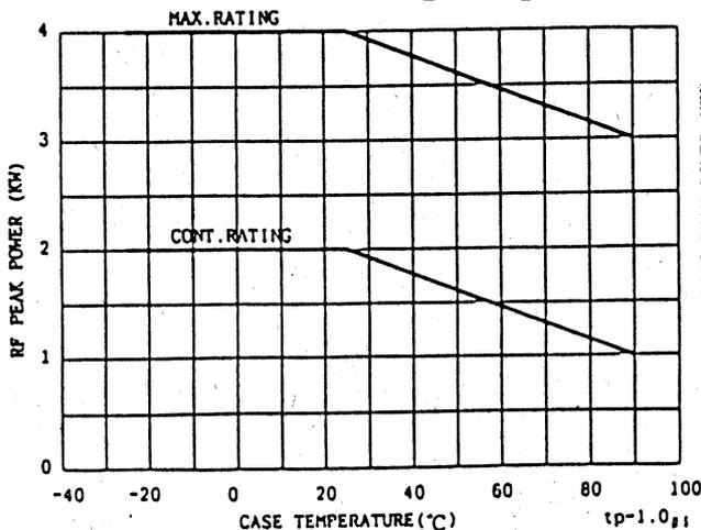
FIG. 1 RF INPUT POWER MAXIMUM AND CONTINUOUS RATINGS
