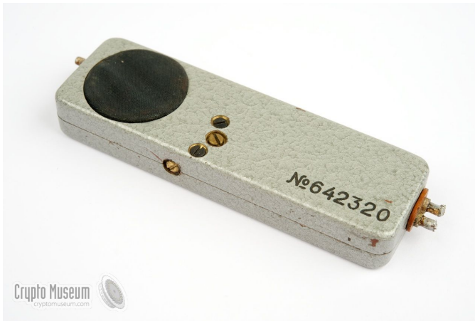
Fig. 3. The KGB Bug, one of the first Soviet transistor-based bugs, created circa 1964. Size 75mm x 23mm x 10mm. Adjustable frequency.
