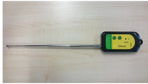
Fig. 15. The Ghost hardware microphone and camera detector. It was used to compare Salamandra against a known working bug detector.
