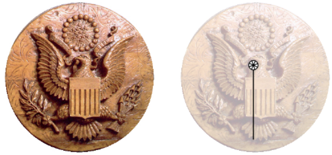
Fig. 2. The Great Seal Bug, also known as The Thing, was a passive listening device invented by the Soviet Union at the end of the Second World War.
