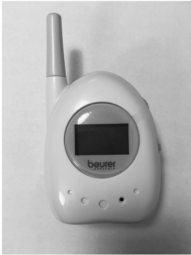
Fig. 10. The Beurer BY 04 is an audio monitoring device designed to monitor babies that operates in the 864 MHz. Size 6cm x 4cm x 11cm. Anyone with a receiver in that frequency can listen to its transmission.
