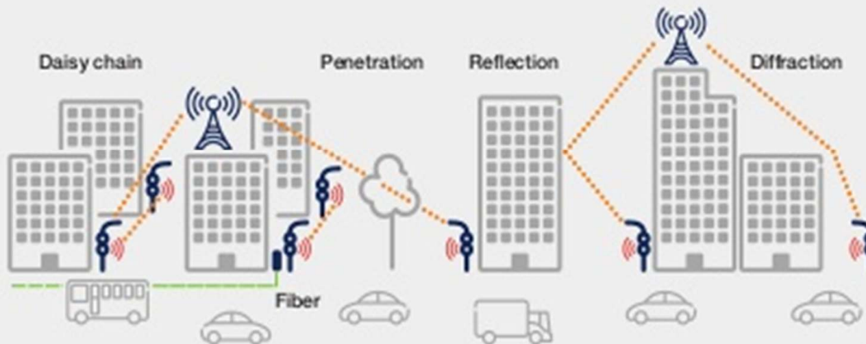
FIGURE 1 Microwave backhaul scenarios for small-cell deployment
