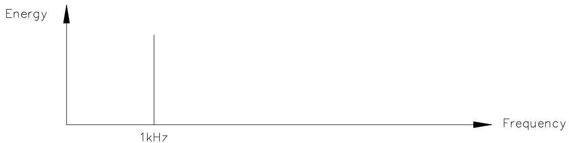
Figure 5-4: Power Spectrum of 1 kHz Sine Wave
