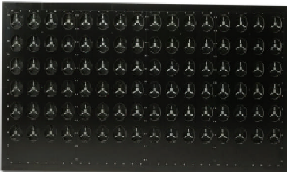
Sample 96-Microphone Array Configuration.....
