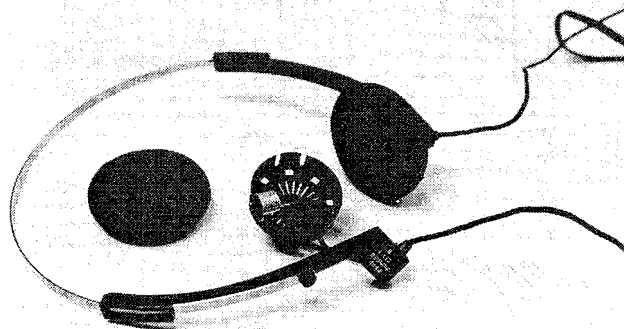
A microphone capsule fits neatly into the space that's left when the speaker element is removed from the earpiece of a miniature (lightweight) stereo headset.
