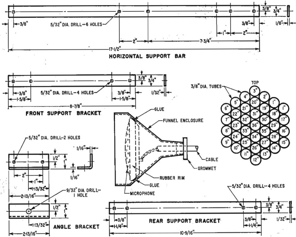
Easily worked aluminum is used for fabricating the pickup. The tubes can be conveniently cut from ten 6' lengths of 3/8" diameter stock, the support bracket-
