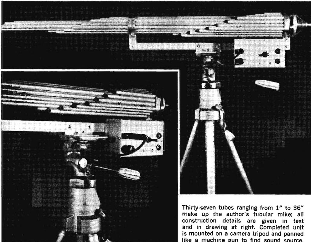
Thirty-seven tubes ranging from 1" to 36" make up the author's tubular mike; all construction details are given in text and in drawing at right. Completed unit is mounted on a camera tripod and panned like a machine gun to find sound source.
