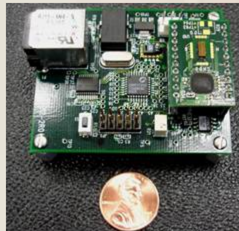
Microsensor Array monitors CO 2 , humidity, temperature, and room occupancy
