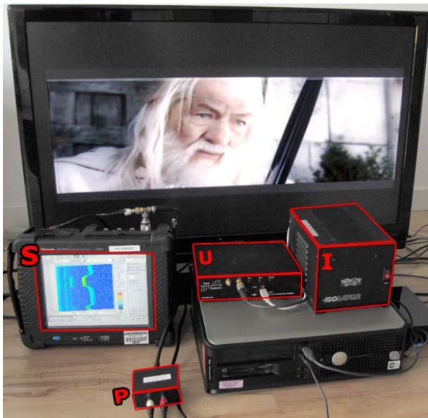
Figure 2: Components of our EMI capture hardware: Power Line Interface (P) for filtering 60 Hz signal voltage sensing, high speed digitizer (U) for analog to digital conversion of signals and an isolation transformer (I) for filtering EMI from other devices in our laboratory environment. The Sharp 42” LCD TV and the data logging PC are also visible. We also connect a spectrum analyzer (S) for debugging purposes and for visualizing the real-time EMI signal as a waterfall plot.
