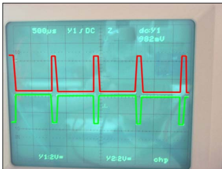
The original signal (green, -3\text{V} ) and after amplification (in red, +5\text{V} )
