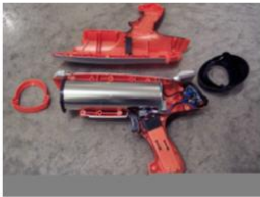
Fig. 19 Inside of Mattel Radar Gun
