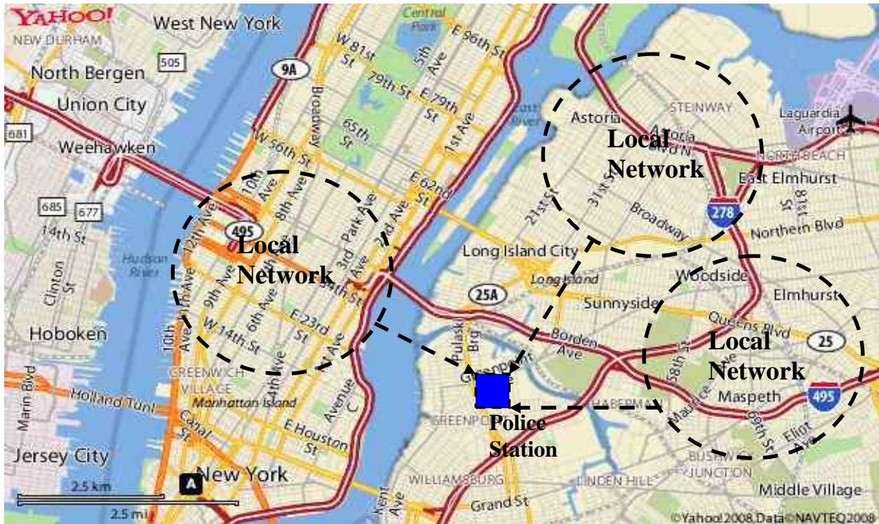
Fig. 50 LPR application of networked LPR/SD systems in a hierarchical star shaped network
