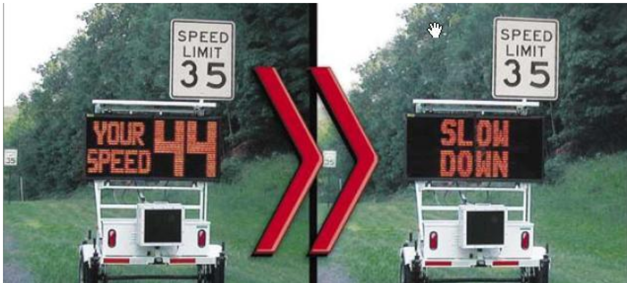
Fig. 47 Example of variable message traffic displays
