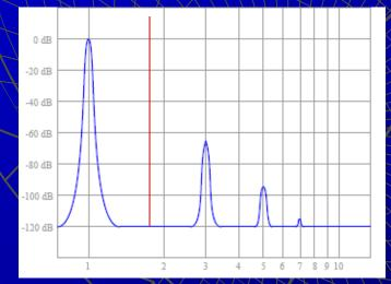
$$v_{square} = \frac{4}{\pi} V_m \left( \sin \omega t + \frac{1}{3} \sin 3\omega t + \frac{1}{5} \sin 5\omega t + \frac{1}{7} \sin 7\omega t + \dots + \frac{1}{n} \sin n\omega t \right)$$
