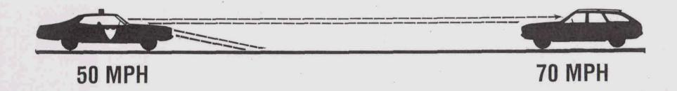
1 CONTINUOUS BEAM OF ENERGY IS SENT OUT 2 DOPPLER SIGNALS ARE RETURNED 50 MPH SIGNAL "GROUND" SPEED 120 MPH SIGNAL "TARGET" SPEED
