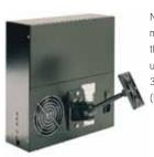
Note: The bracket mounting bolts on the rear of the HSS unit require USA 10-32 Nuts (metric M5 (5mm - 8)).
