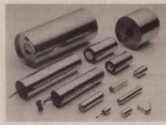
Battery Engineering Lithium-Thionyl Chloride batteries can be made in virtually any shape with packages and electrode structures designed to customer requirements. Featuring 200 Whr/Kg energy density and discharge capacities from .06 to 135 amp-hours, they retain up to 80% of their original capacity after 10 years.
