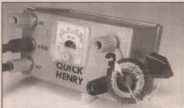
The unknown inductor is connected to the "?" binding posts, and a parallel capacitor selected.
