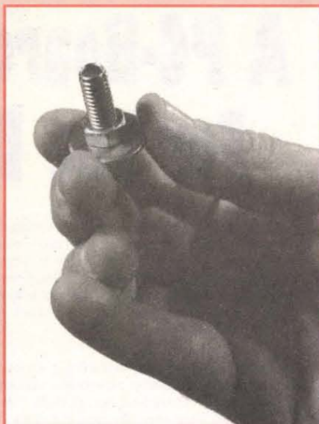
Figure 5. Carriage bolt and nut assembled for soldering.
