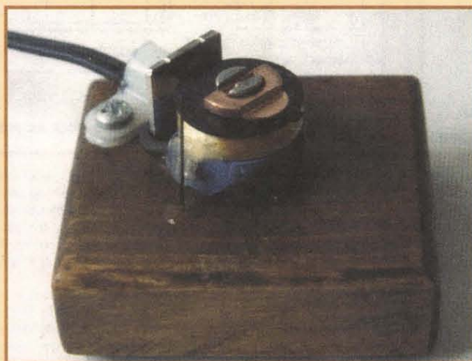
MODEL OF FLEMING & THOMSON MOTOR WITH ROTOR REMOVED
