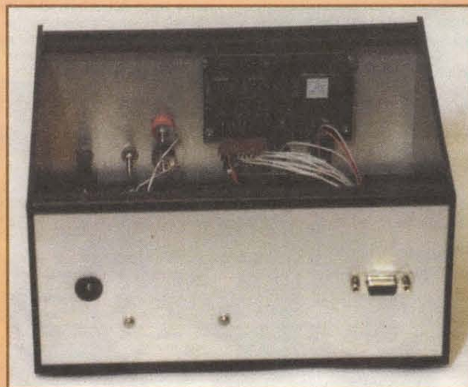
Figure 8. Photo showing the LCD display which is attached to the front panel with four 2-56 x 1/2 inch machine screws, nuts, and 1/4 inch long spacers. Place a nylon washer between the spacer and LCD board for insulation and to add 1/16 inch to the spacer length. The rear panel shows the power input connector on the left and serial DB9 on the right.
