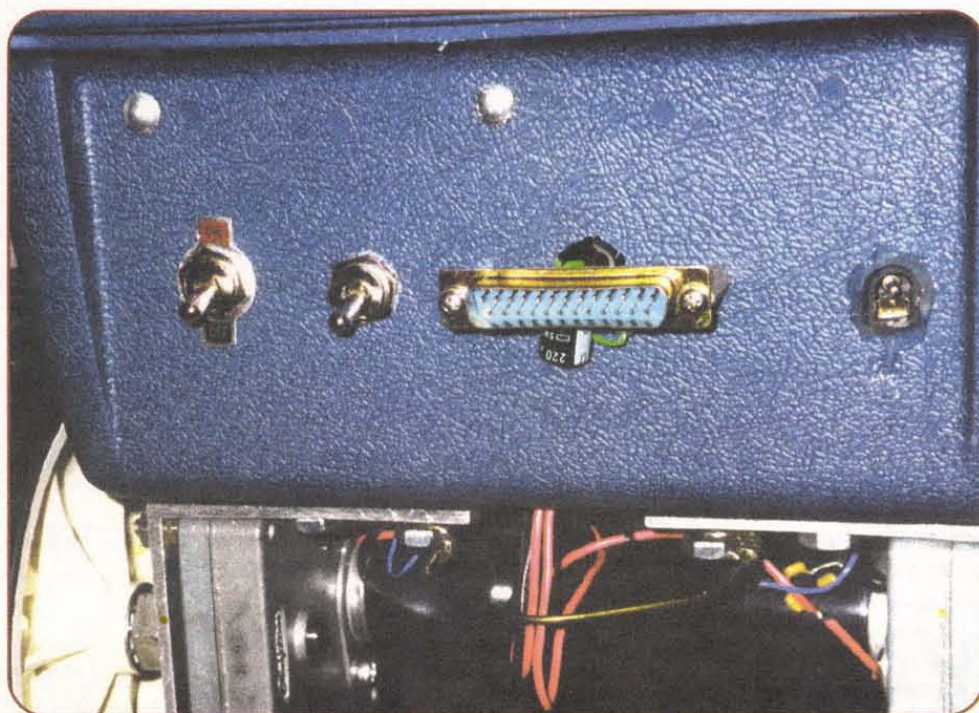
A look at Tacklebot's rear apron, showing the main power switch, motor power switch, DB-25 tether connector, and battery charger jack.
