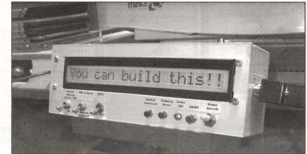
Figure 6. Operational MMM Displaying Interpreted RS-232
