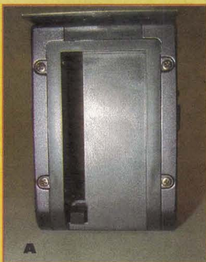
Figure 3. a) PC Card slot at rear of body, and b) LCD display and controls on front.
