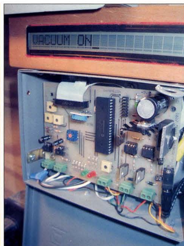
Figure 17 Completed/ Installed DUSTMEISTER (Access door open)
