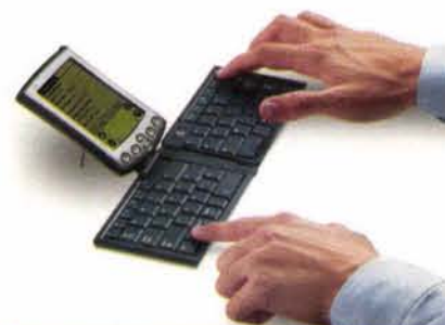
The Logitech TypeAway™ keyboard extends input capabilities of Palm handhelds via the Palm Universal Connector. Photo courtesy of Logitech International.
