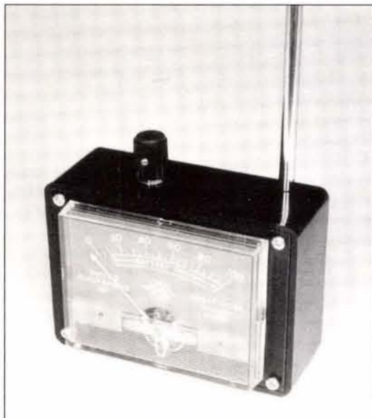
The completed RF Meter sensitivity is controlled by a top-mounted knob.
