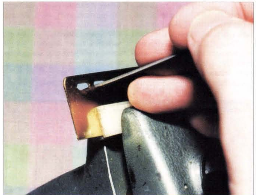
PHOTO 4: Filing the limit switch adjustment slots on the mounting tab.
