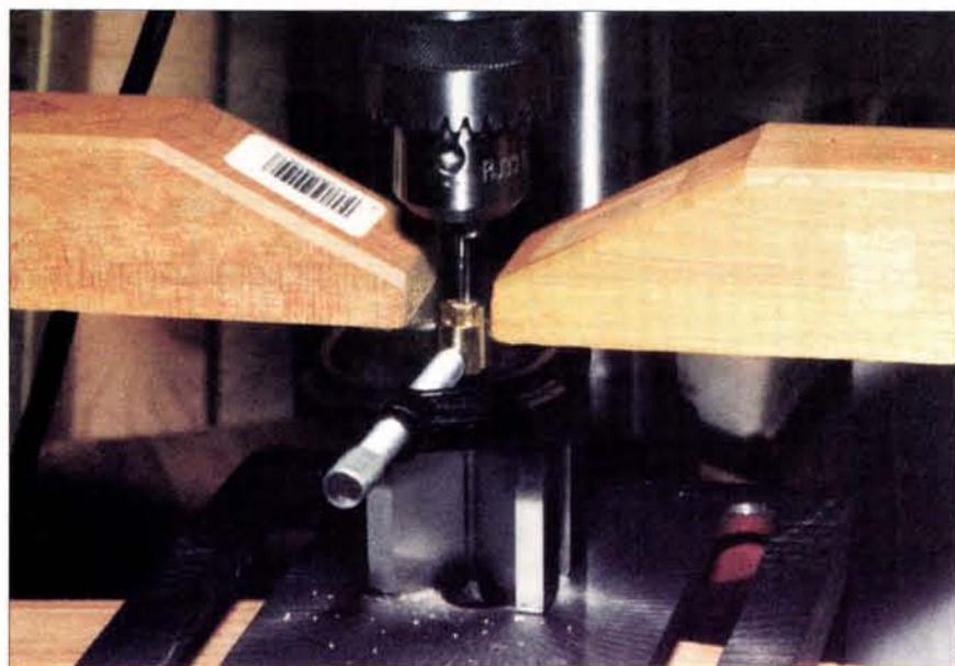
PHOTO 1: Clamping arrangement for drilling and tapping the follower nut. The V-block holds the block in alignment with the drill press spindle, and the wood clamps keep the V-block from moving. Adjust side-to-side and back-and-forth with light taps from a mallet handle.
