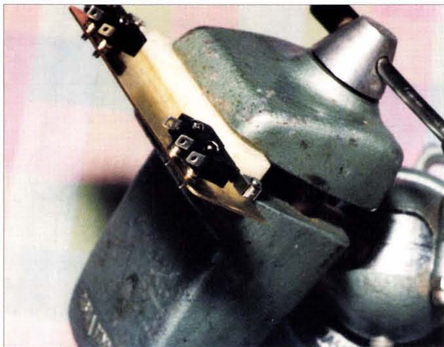
PHOTO 5: The limit switches on the mounting tab. Use #2 washers to space the switches up from the tab so their rollers are aligned with the centerline of the slide assembly.
