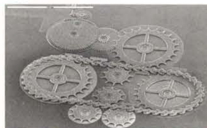
Sandia's microchain can provide space reduction in powering MEMS devices. Courtesy of Sandia National Laboratories.
