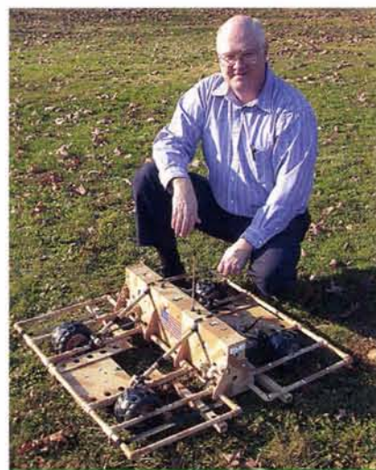
The Mine Rover, developed at Johns Hopkins University's Applied Physics Laboratory, provides sophisticated, inexpensive mine detection. Photo courtesy of Johns Hopkins APL.
