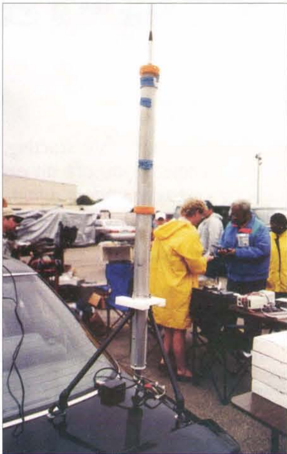
Trunk lid ground for this big coil whip.
