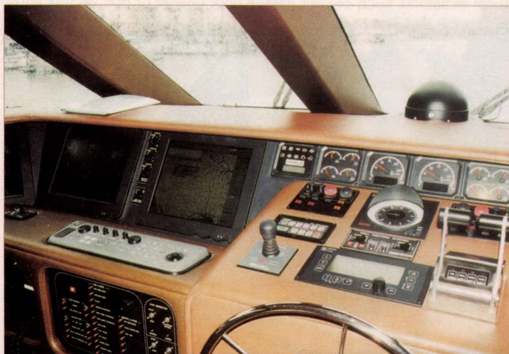
Noise from the refrigeration controller wiped out this super yacht's long-range radio reception.
