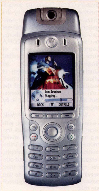
FIGURE 2. Many 3G and even 2.5G phones have built-in digital camera and/or video capability. The camera eye at the top of the unit digitizes your picture and transmits it while you can display the caller's photo on your color LCD screen. This is Motorola's A820 3G phone. Courtesy Motorola.
