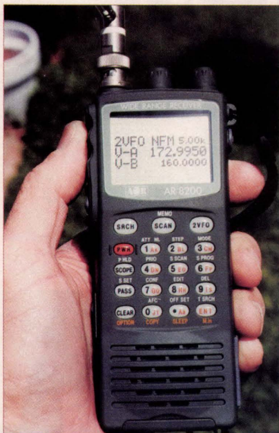
The AOR "noise sniffer" in action showing noise indications on the LCD display.
