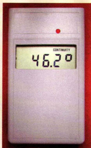
Figure 9. The measured angle is displayed on the LCD as degrees in tilt-angle meter mode.
