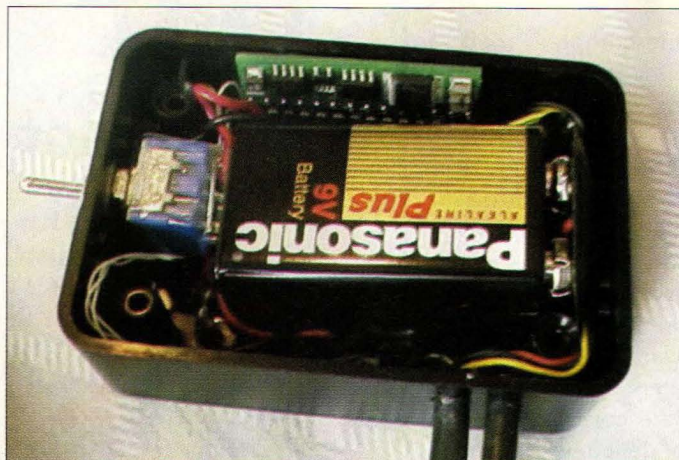
Figure 5: The internals of the computer module, including power switch (left), BASIC Stamp computer (top), and battery (center). Wiring is routed around the perimeter of the module.
