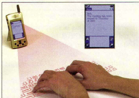
Canesta's chipset will allow full-size projection keyboards to be incorporated in mobile devices. Courtesy of Canesta, Inc.
