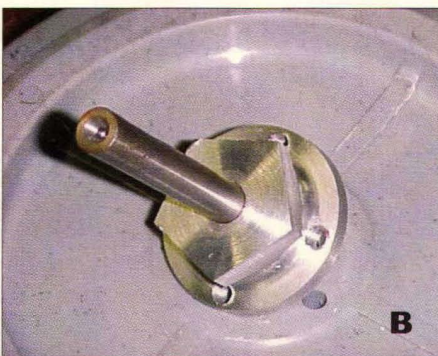
Figure 2. Custom Hub and Axle Parts A and B. Part A shows the round side of the hub with the bolt pattern. This end is secured in the wheel by four bolts. Part B shows the pentagon-shaped hub that mates with the pentagon-shaped drive piece of the motor. The axle is made of steel and is pinned to the aluminum hub. This had to be made on a milling machine and a lathe. Purchased at Wilson's Welding of Linwood, NC — you should be able to find a local machine shop that can do the job.
