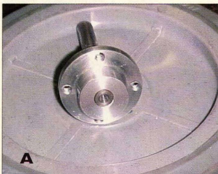
Figure 2. Custom Hub and Axle Parts A and B. Part A shows the round side of the hub with the bolt pattern. This end is secured in the wheel by four bolts. Part B shows the pentagon-shaped hub that mates with the pentagon-shaped drive piece of the motor. The axle is made of steel and is pinned to the aluminum hub. This had to be made on a milling machine and a lathe. Purchased at Wilson's Welding of Linwood, NC — you should be able to find a local machine shop that can do the job.
