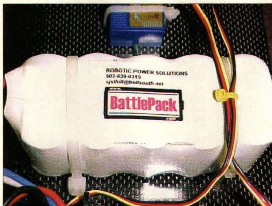
Figure 4. Battlepack Batteries. Shows a 12-volt battery pack. The speed controllers I chose can only handle up to seven cells, so a custom pack will be necessary. I modified the pack myself so that I can use it again on a later project at the original voltage. Purchased at www.battlepack.com , custom packs can be ordered at no extra charge.
