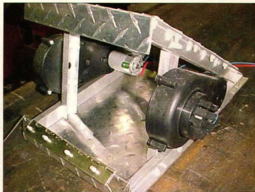
Figure 5. Stick Frame of Wedge Bot. Shows the aluminum "C" channel and armor riveted together. The motors and rear-hinged door are in place too. Materials purchased at the local hardware store.
