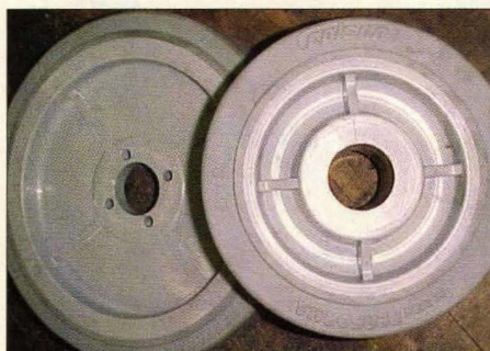
Figure 1. Original and Modified Colson Wheels. Shows two different Colson brand castor wheels. The inner plastic hub is very sturdy. The outer layer of rubber is a good match for traction and strength. The large wheel has been modified with a milling machine to make the plastic hub thinner for a better fit on the custom axle for this particular bot. The small wheel has not been modified and will be used on a different project. Before modification, the hubs on both wheels are similar. Can be purchased at www.botparts.com (Part #BPDWC20) or www.teamdelta.com (Part #RCM307).
