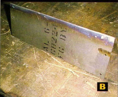
Figure 2. Titanium Armor. Part A shows the titanium in its original shape. Part B shows the titanium after bending. When bending this metal, heat it with an oxy/acetylene torch in a straight line until red hot. The material is so thin that it will warp. While it is red, use a press brake to bend it into the shape of the tip of the wedge. Do not let it cool before bending or it will snap. The press brake will also flatten the warp.
