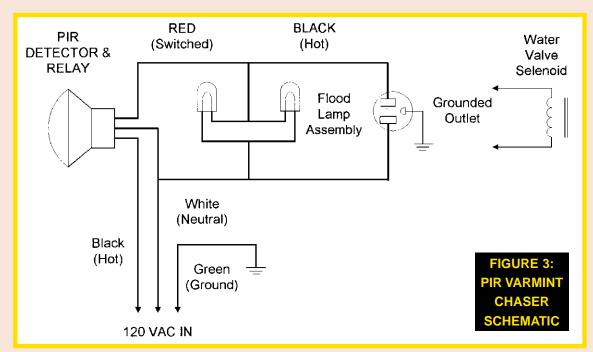
vicinity to be protected. The solenoid valve does not have to be attached to anything. Finally, using double-female washing machine supply hoses, connect the input of the solenoid valve to your hose bib, and the output to a garden sprinkler.
