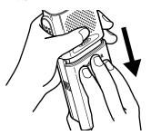
With the battery label facing up, align the contacts on the battery pack with the contacts inside the battery compartment. Then press the battery pack into the compartment while applying slight pressure to the bottom of the battery pack.
