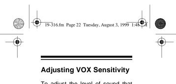
To adjust the level of sound that activates transmissions, set **VOX** to **ADJUST**.
