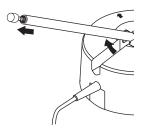
**Note:** Fully extend the antenna for maximum range.
