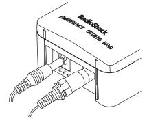
2. Ensure the cigarette-lighter plug cap is tightly screwed onto the plug and insert the plug into the cigarette-lighter socket.
