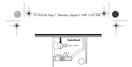
If the indicator lights, the batteries are good. If the indicator is dim or does not light, the batteries are weak or dead and need to be replaced.
