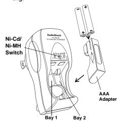
To charge four Ni-Cd or Ni-MH AA batteries, install two batteries into each bay as indicated by the polarity symbols (+ and -) marked inside each compartment, then slide Ni-Cd/Ni-MH to the appropriate setting.
