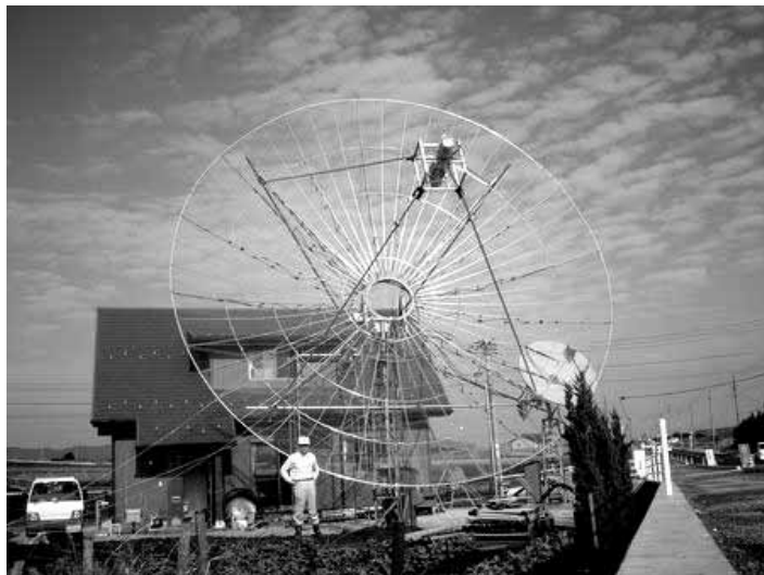
The impressive Japanese EME station at JR4ZZS with 9m dish and 23cm feed. The operator pictured here is JR4AEP
