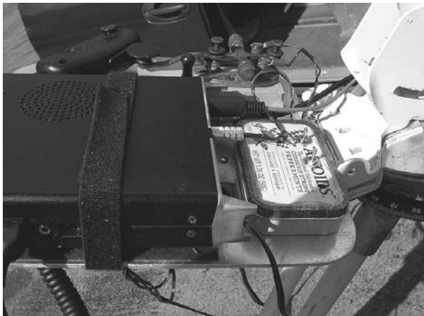
Figure 1: The Dash-Sender in the Altoids box keying my FT-817 in the 10 GHz contest 2006
