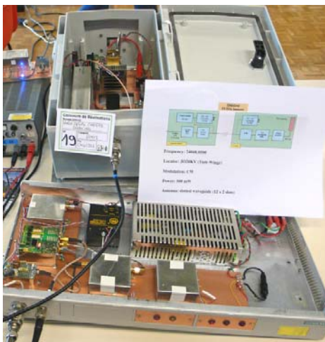
Above: ON0GHZ beacon hardware on display at CJ2009 . Indoor unit in the foreground, with the masthead box at the rear.
