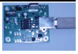
grated frequency synthesizer, with steps and resolution to 1Hz. The Si570 is programmable via an I2C interface and the kit includes a ready programmed ATMEL AVR to connect via USB to PC/ free software. All components, less enclosure and connecting cable, are included in the kit. This includes a good quality plate through hole (PTH) PCB. Components are a mixture of surface mount and leaded components.
