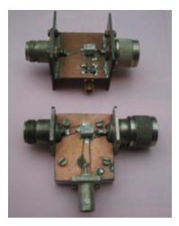
Although having a good selection of test gear, I do not have a signal generator that covers 1-2GHz. To overcome this problem, I have used a JMS.2411 mixer from a redundant Ionica unit and I have modified a G4DDK board using a 83.333Mhz crystal to give an output at 1GHz. This is fed to one port of the mixer and then I can use my 0-1 GHz signal generator on the other port to mix with it to give me 1-2GHz.
