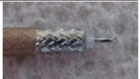
Figs. 4,5 – RG316 cable preparation
