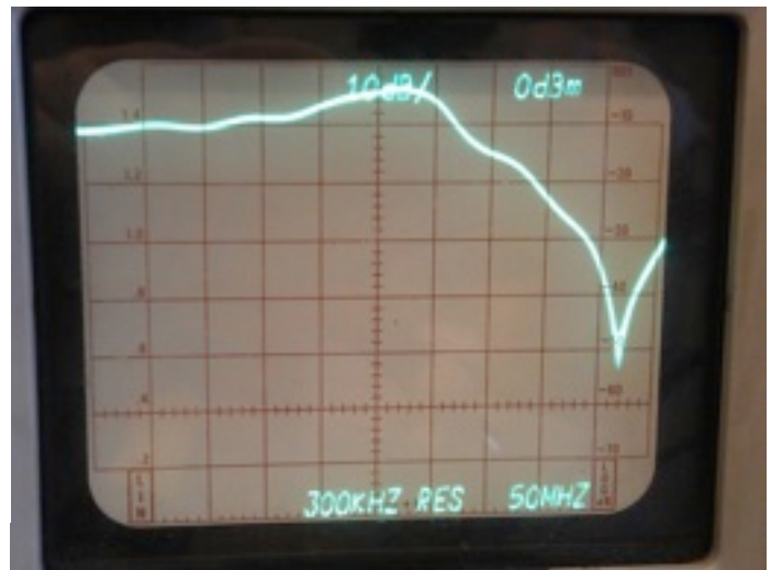
Fig. 4 – Measured Gain of Preamp and Filter. Centre Frequency 1090MHz, 0dB gain is at the -20db line, 50MHz/div, 10dB/div.
