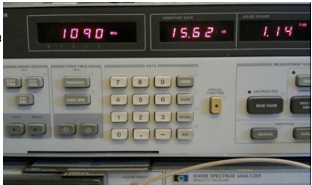
Fig. 6 – Gain and Noise Figure measurement.
