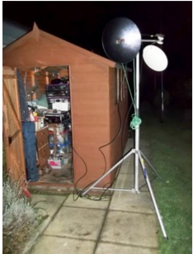
G6GVI, scattering off a wall behind the camera. The black dish with “penny-feed” is for TX and the offset dish & LNB for RX
