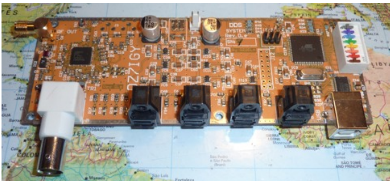
Digital synthesizer with USB control port.
