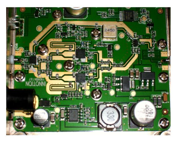
From the data they give a claimed 1dB compression of 34dBm. Supply current peaks around 1.15A. There is an on-board switch mode supply, so 10 -14V is fine.
