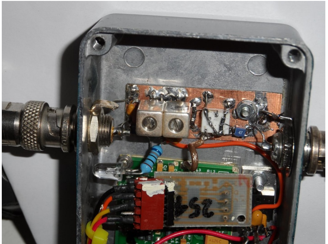
Photos 1 and 2. Two Views of the finished LNB Downconverter. The LMX2541 Fractional-N synthesizer module is shown partially concealed below its PIC controller PCB
