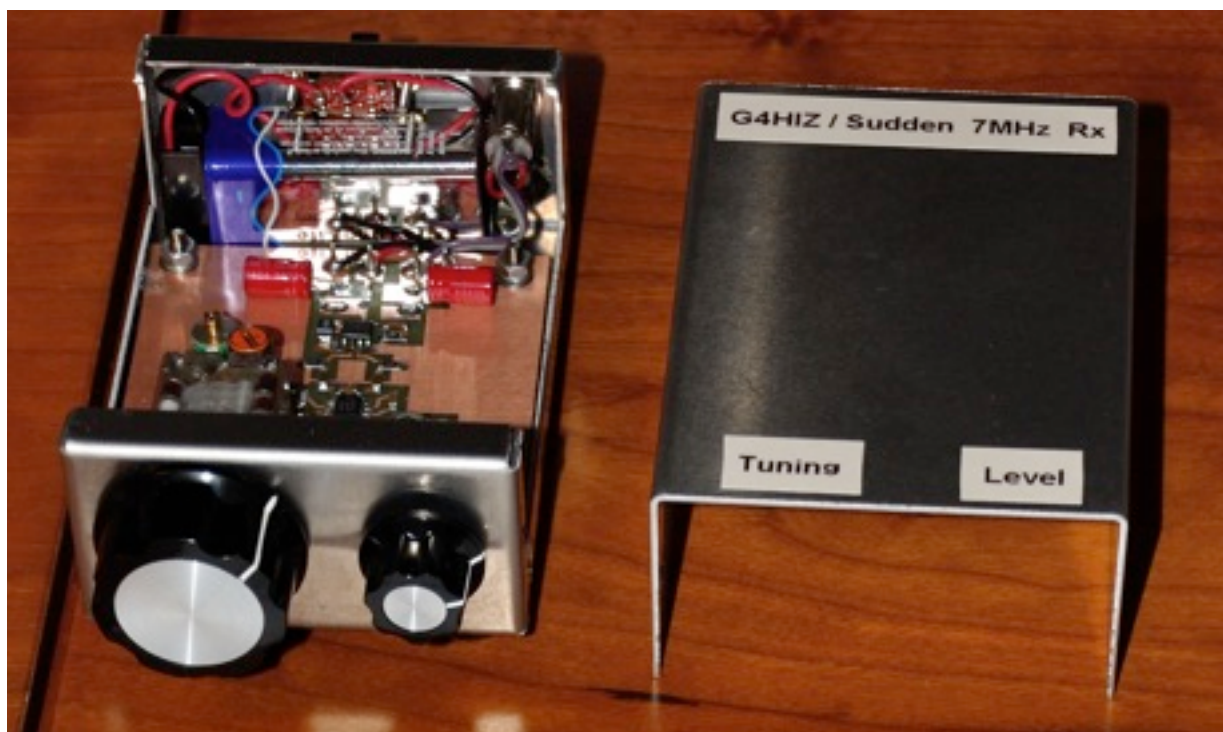
"A good accessory for the serious microwaver" A 7MHz CW practice receiver using SM components by Jeff Eastdown G4HIZ
