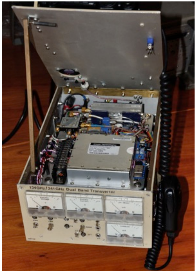
Right: 134 / 241GHz transverter system by Chris Whitmarsh G0FDZ
